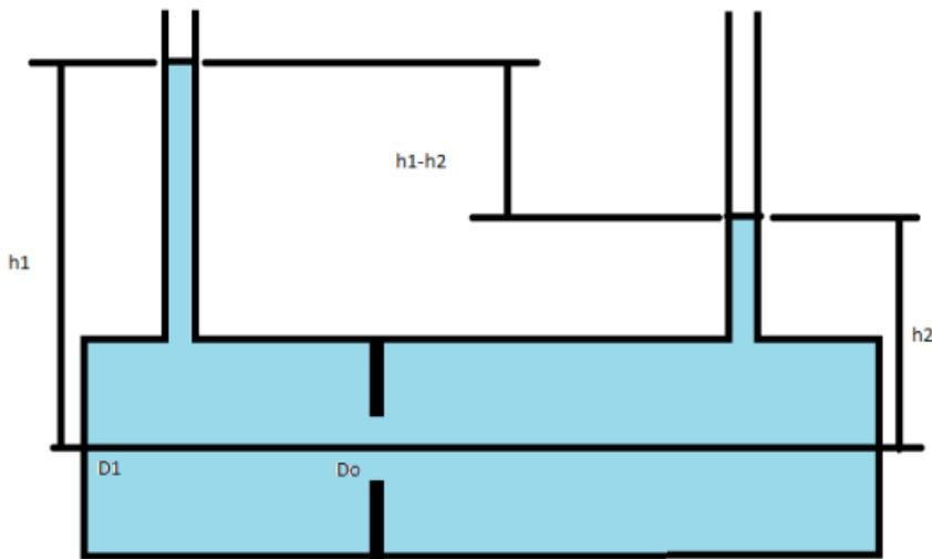
**Fig 4.10** Orifice Plate
