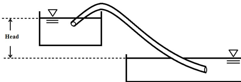
Fig. 4.11 Measurement of Head for Siphon Tube
