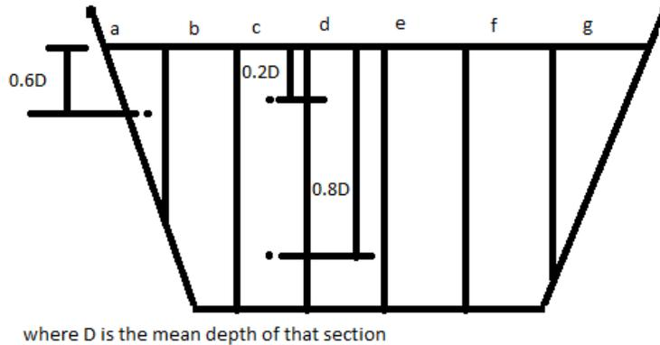
**Fig. 4.3** Measuring Points in Channel Cross Section
