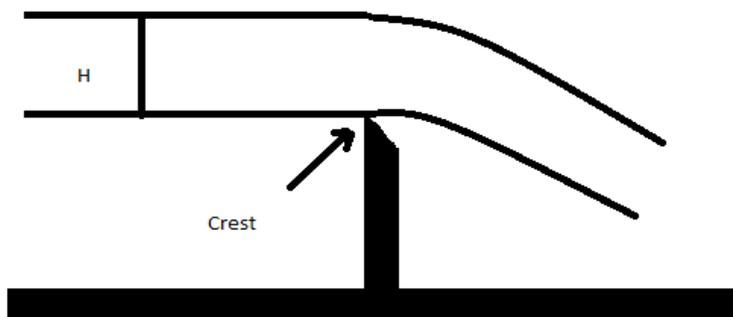
Fig. 4.5 Water Flowing Over a Sharp Crested Weir
