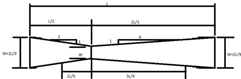
**Fig. 4.7** Sketch of Cutthroat Flume (Top View)
